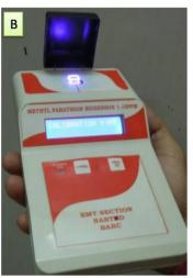
Figure 5B. Handheld colorimetric biosensor for detecting methyl parathion
