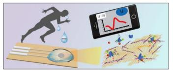
*Fig 1: Silk-Based Electrochemical Sensor for the Detection of Glucose in Sweat (Reproduced with permission from ref. 8. Copyright (2022) American Chemical Society)*
