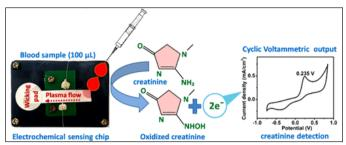
*Fig 4: Schematic diagram of reduced graphene oxide based creatinine detection (Reproduced with permission from ref. 11. Copyright (2021) American Chemical Society)*
